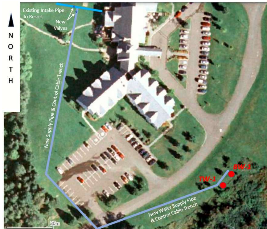
Figure 6. Route of trenching for new water supply pipe and controls cable from new production wells to existing intake pipe into Resort building. Valving was also installed on the existing intake pipe as well as the new supply pipe.
