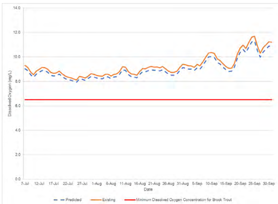
Figure 3.2 Calculated Minimum Baseline and Operational Dissolved Oxygen Concentrations (mg/L) in Forty Mile Brook, NB
