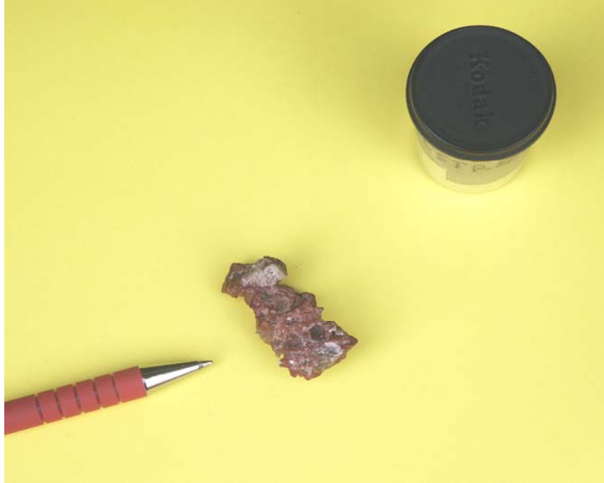
Figure 2. A 4-cm long potash (sylvinite) fragment from the Millstream # 1 discovery well drilled by the New Brunswick Department of Natural Resources in 1973.
