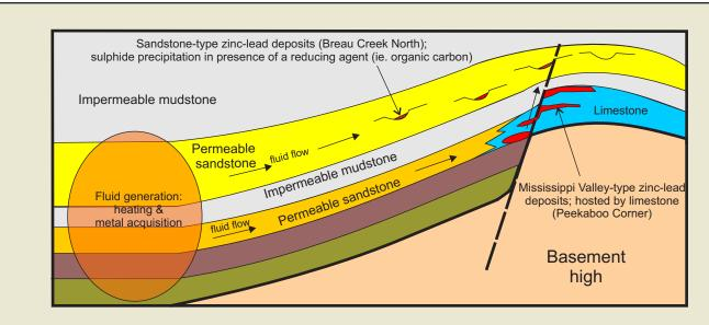
**Figure 5**. Conceptual model for the generation of sandstone-type and Mississippi Valley-type zinclead deposits, with New Brunswick examples. Compiled from Graves and Hein (1994), NBDEM (2013), and Sangster (1996a and b).
