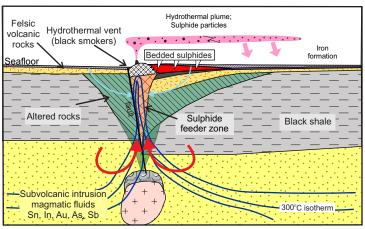
**Figure 3**. Model for the formation of volcanogenic massive sulphide (VMS) deposits. Modified from Goodfellow (2007).
