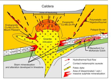
**Figure 4**. Model relating endogranitic, polymetallic vein, and skarn zinc mineralization to granitic intrusions with examples cited in text. Note that a significant example of an exogranitic zinc deposit has not been identified in New Brunswick.
