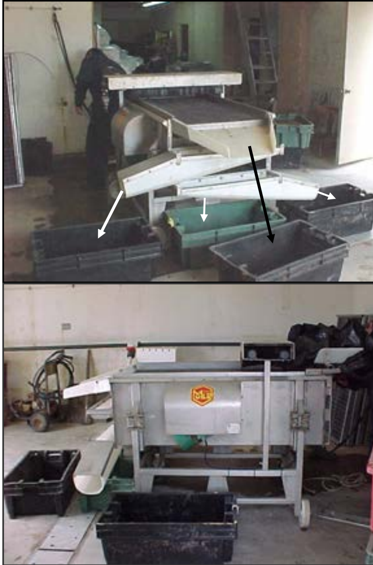
Figure 29 Vibrating screen (commercially manufactured)
