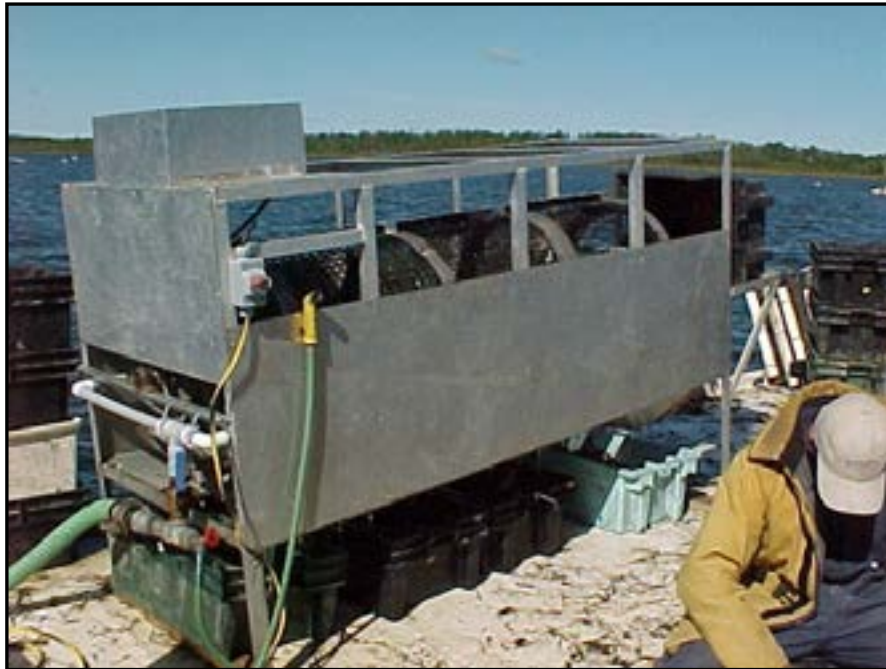
Figure 28 Oyster sorting machine (home-made)
