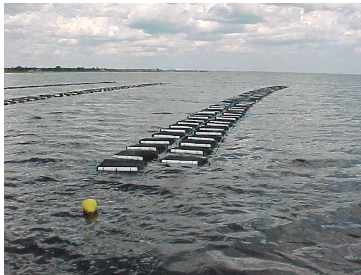
Figure 4: Longlines of floating bags on the Saint-Simon Sud site
