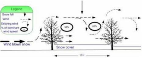
Figure 2. A porous windbreak will distribute snow evenly.
